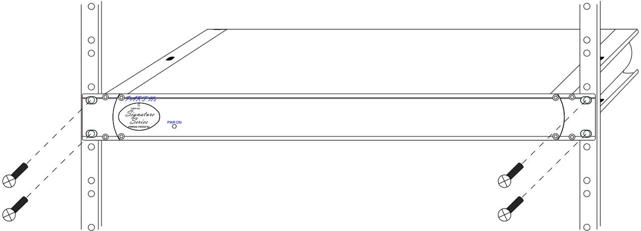
Firmly hold the signature subrack within the 19" rack and locate in 1RU of space. Use the supplied 6mm rack screws to securely attach the unit to the rack.
