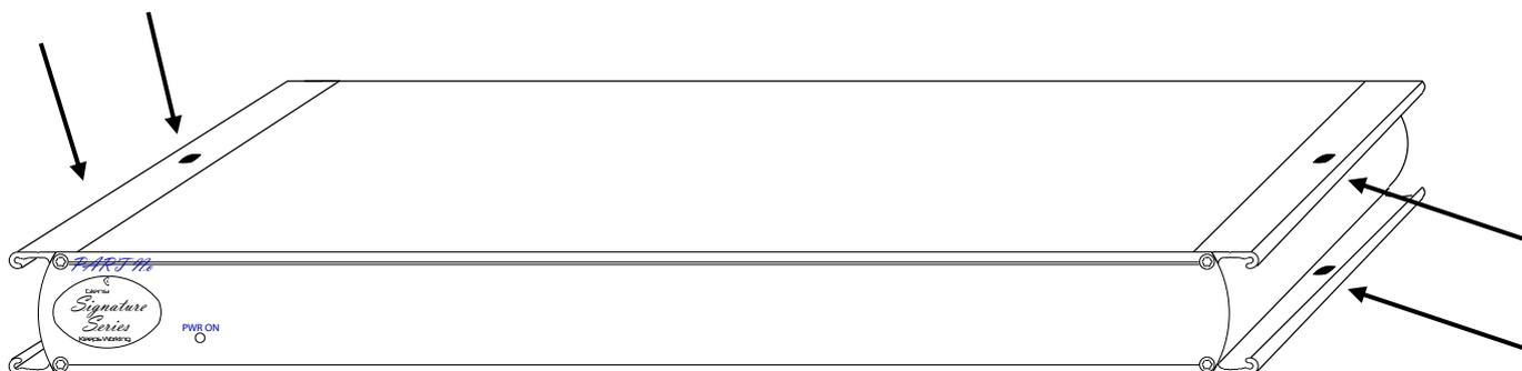
Use either the top or bottom mounting holes as indicated above to use suitable screws to attach the signature unit to a worktop or bench. **\*\*PLEASE ENSURE THAT YOU USE SUITABLE FIXINGS\*\***
