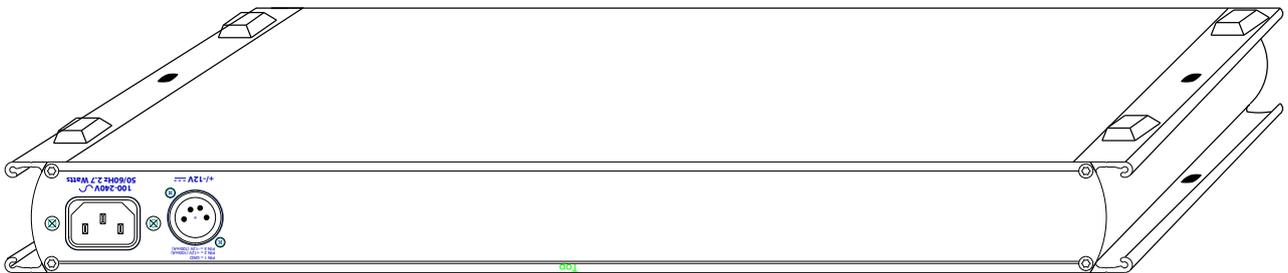
Remove the front rack ears (if they are not required), turn the unit upside down and attach the supplied 4 sticky feet as per the above drawing.
