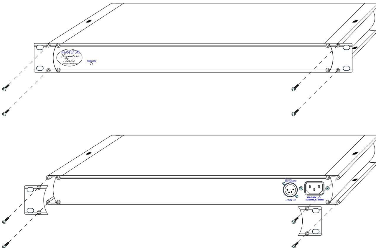
First remove the 4 silver button head screws that fix the rack ears onto the front of the unit as shown in the top picture above.
